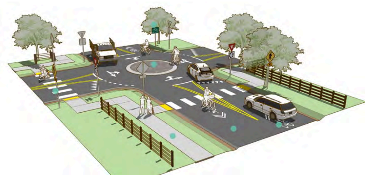
Figure 20 - Bicycle Boulevard & Intersection (Source: Small Town & Rural Design Guide)
